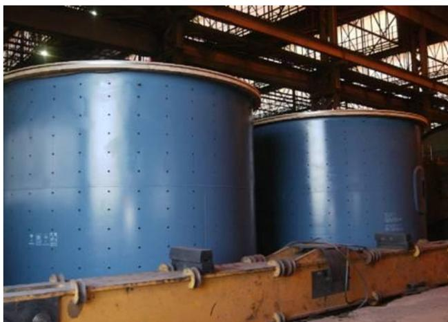
**Figure A – Ball mill shells completed and in storage in Singapore**
