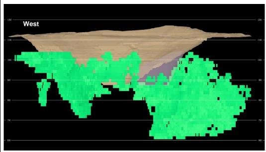
Figure 3.5 Martha Underground Mineral Resource Long Section
