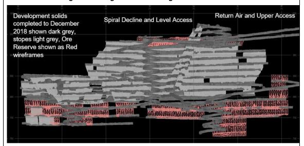
Figure 4.2: Long Section of Underground Ore Reserve
