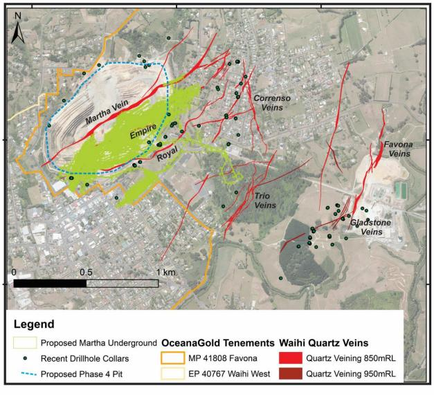
Figure 2: Maps showing WKP Location and Drilling
